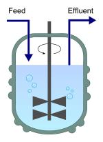
Constant volume. Substrate pumped in and substrate/biomass mixture pumped out at same rate
