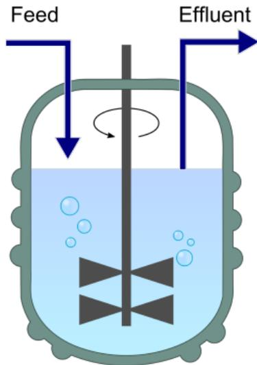
Constant volume. Substrate pumped in and substrate/biomass mixture pumped out at same rate
