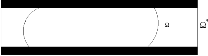
Fig. 1. The basic configuration of an electro-wetting on dielectric device. The solid black region depicts the dielectric plates and the white region denotes a droplet of one fluid (say water), which is surrounded by another (air). We denote by \Omega the fluid domain, by \Gamma its boundary, by \Omega^* the region occupied by the fluids and the plates and by \partial^*\Omega^* := \partial\Omega^* \setminus \Gamma .
