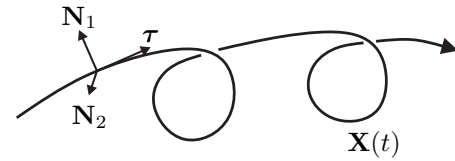
(a) Curve parametrization; \tau is the tangent vector of \mathbf{X} . The triplet \{\tau, \mathbf{N}_1, \mathbf{N}_2\} is an orthogonal frame.
