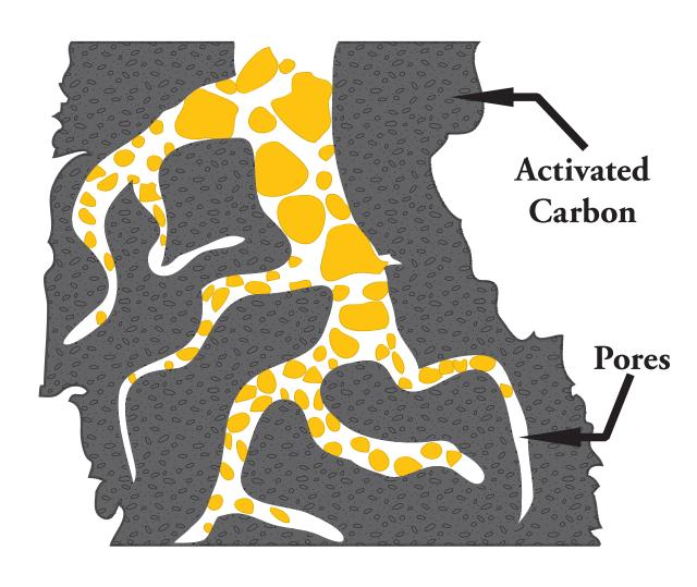
The GAC filter passively controls and regulates the flow of pollutants. The submicroscopic pores trap pollutants through a process called adsorption. As non-contaminated liquid or air flows through the filter, the granulated carbon releases stored pollutants.
