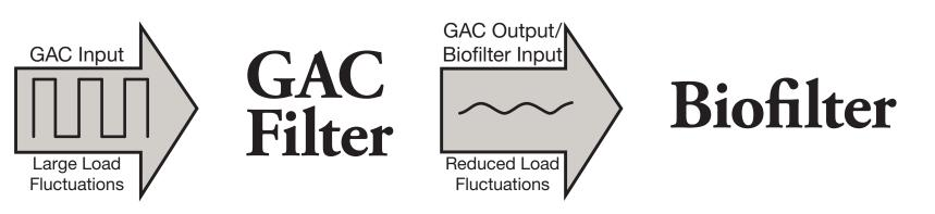
A GAC filter is able to stabilize loads passively due to its ability to both adsorb contaminants during periods of increased loading and desorb previously adsorbed contaminants during periods of reduced loading. The GAC filter will initially adsorb practically all contaminants until it has reached a quasi-steady state breakthrough. It then begins to have an output in correlation with its input and it also acts to attenuate changes in the contaminant loading.
