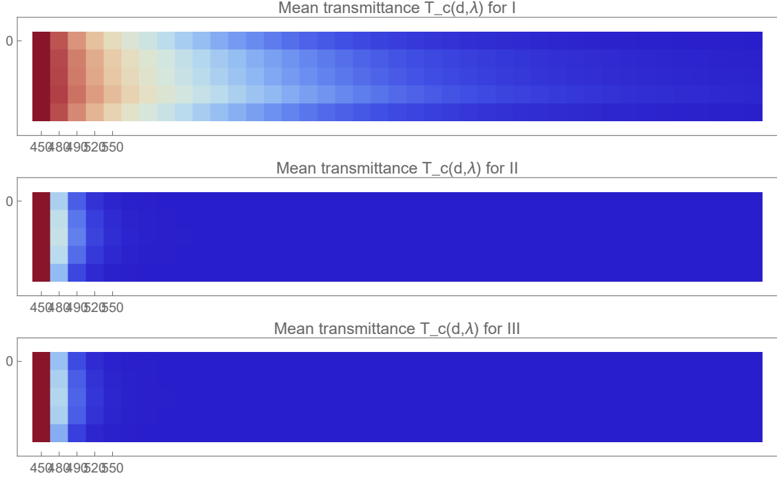
Figure 3: Heatmaps of mean T_c(d, \lambda) across distance and wavelength for representative Jerlov types.
