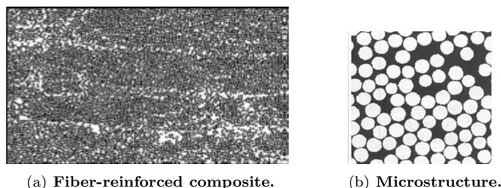
Figure 1: **Fiber composite and microstructure.**
