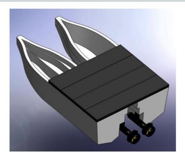
Victoria's hull was made of s-grade fiberglass and a super hard epoxy resin, with a 1 to 1 weight ratio between glass and resin. A vinyl-epoxy white sealer was used as a final layer. The two hulls in the catamaran-style design have room to house the batteries and electronics, leaving space for sensors on the platform that joins the two hulls together.
