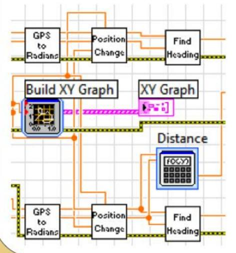
NI LabVIEW 2011 was used to program both the CompactRIO on Victoria as well as the user interface running on the control laptop back on shore.
