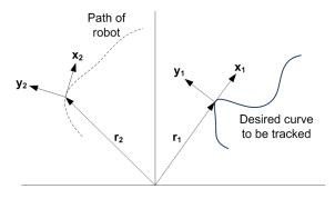
Simpler 2D case: Boundary following with gyroscopic control.
