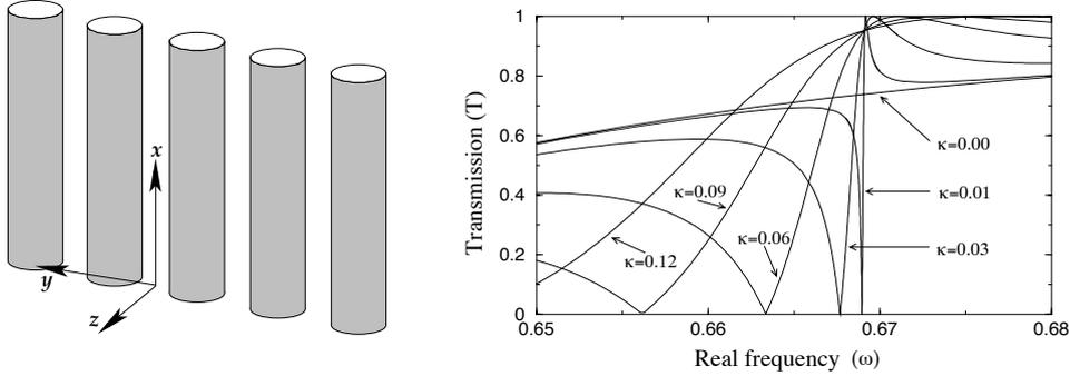
Fig. 2. Transmission of  $E$ -polarized EM fields through a periodic array of infinitely tall lossless rods ( $\epsilon = 12$ ,  $\mu = 1$ ) as a function of the reduced frequency  $\omega$ , for various of values of the wave vector  $\kappa$  near the parameters  $(0, 0.669)$  of a guided mode. The exact calculation and the theoretical formula are practically identical.
